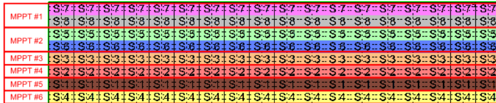
Figure 49: String configuration for Multi-MPPT for both locations
